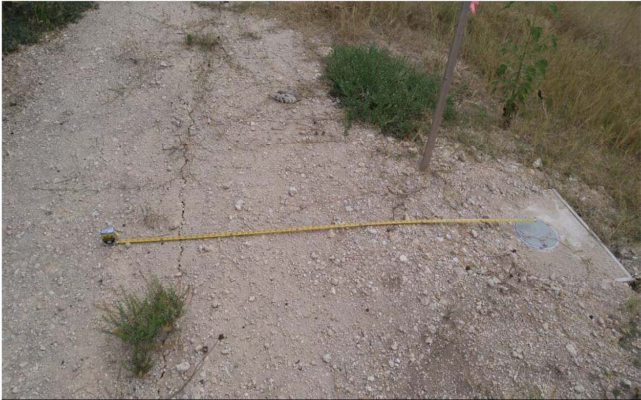
Photo 1 - Looking South - New Surface Tension Crack 5.75 Feet East of ARC-1
